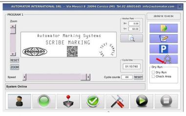
displayed instantly. The software provides for the creation of messages with the date in various formats, fix or variable texts, codes, serial numbers, Datamatrix and logos. Possible the creation of the programs on the PC (running Windows operating systems), which can be easily transferred to the AC500 controller with USB stick or USB connection.
